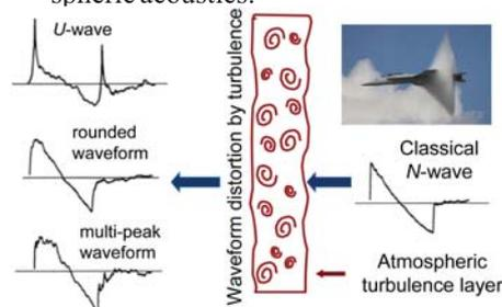
Fig. 2. Propagation of nonlinear waves in randomly inhomogeneous media. Application: sonic boom problem. Aircraft, while moving supersonically, generates an acoustic shock wave, which is called sonic boom. Propagating further to the ground the acoustic waveform is distorted by the atmospheric turbulence.
