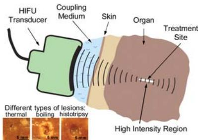
Fig. 1. Focusing nonlinear ultrasound waves in biological tissue. Application: High Intensity Focused Ultrasound (HIFU) surgery. The transducer radiates a focused ultrasound beam through the overlying tissue layers to create a high intensity region within the organ and induce thermal and/or mechanical damage of tissue.
