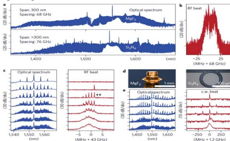
Wide optical spectra of optical combs in  $MgF_2$  and  $Si_3N_4$  microresonators (a). Broadened RF beatnote signal for  $MgF_2$  cavity (b). The evolution of optical and RF beat spectra in  $MgF_2$  and  $Si_3N_4$  (c,e) resonators shown (d).
